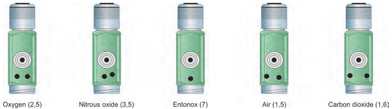
Fig. 2.6: Pin index safety system for different gases. Two pins in the hanger yoke of anesthesia machine are aligned with two corresponding holes on the cylinder head in order to prevent mounting of a wrong cylinder. Exception being entonox which has one pin on yoke and corresponding hole on cylinder.
